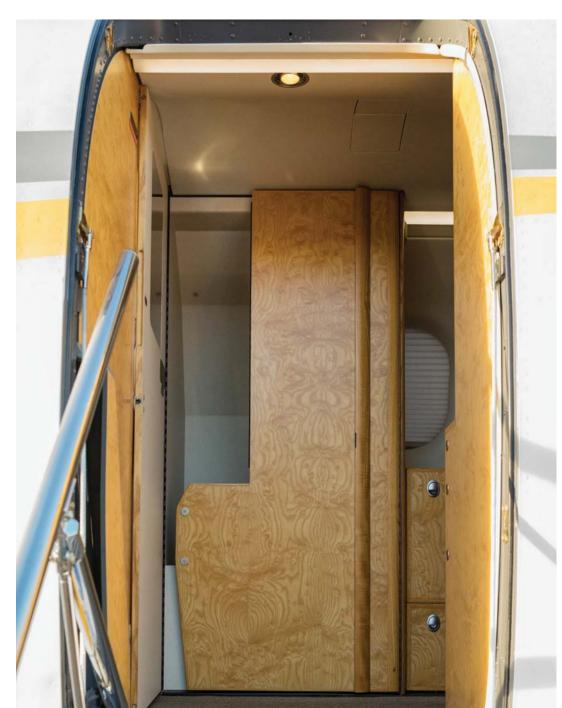
Enclosed Lavatory unit oppposite entry door Hardwood Privacy Dividers Chemical Toilet Drop-down Oxygen Mask in the compartment
